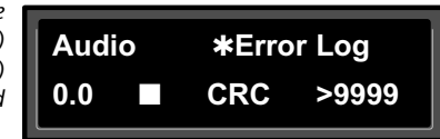
A typical Error Log display showing that the last error received was a CRC error (■ CRC) and that there have been more than (>) 9999 instances of CRC errors since Word Clock was last set to Ext.
